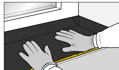
Membrane can be adjusted within 30 minutes after adhesive application.
