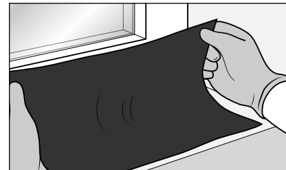
Apply SikaMembran loop-shaped and free from tension.
