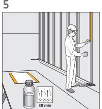
Shake SikaTack® Panel Primer thoroughly (the movement of the steel balls in the container must be clearly audible). Apply one thin coat of SikaTack® Panel Primer uniformly over the whole surface with a felt pad.
