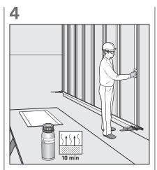
Aktivate the bond faces with Sika® Aktivator-205. Use a clean lint-free paper towel or cleaning paper and wipe in one direction only (dirty cloths must be replaced).
