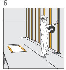
Apply SikaTack® Panel Fixing Tape over the whole length of the vertical sections and parallel to the edges.
