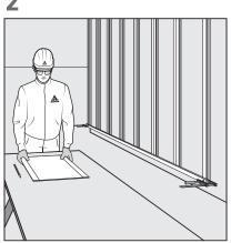
The surface to be bonded must be clean, dry and free from grease. Abrading with an abrasive pad (grain 80) on the panel and the substructure when recommended for the specific system.
